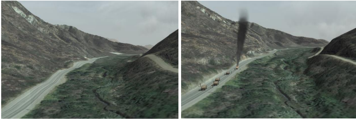
Figure 4 - A comparison of rendered 10m elevation (left) to 1m elevation (right), draped with the same 1ft imagery as displayed in VR-Vantage.
