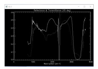
Figure 2. STACK Output for a Water Film over CO2 on a Germanium Substrate at 20K
