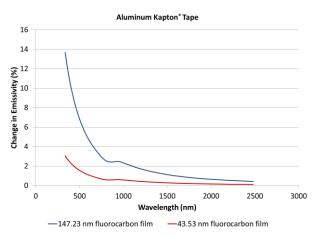
Figure 3. STACK Results for Multiple Film Thicknesses of Fluorocarbon Film on Aluminum Kapton® Tape Substrate
