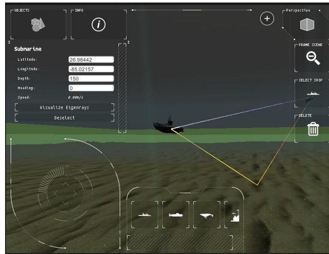
Figure 2. A Perspective View of a Submarine Target from an E-SAIL™ Screen Capture Showing Integrated Display of Eigenray Data for that Target.
