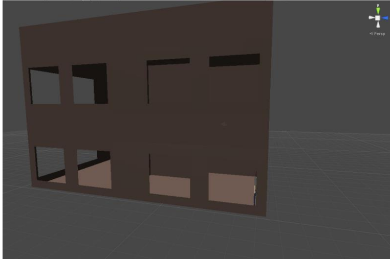
Figure 4: Revit file for FRP2 after import and a light object added. Due to format differences and file conversion losses, the walls are flat planes, have no textures applied to them, and have no colliders for physically-realistic interaction.
